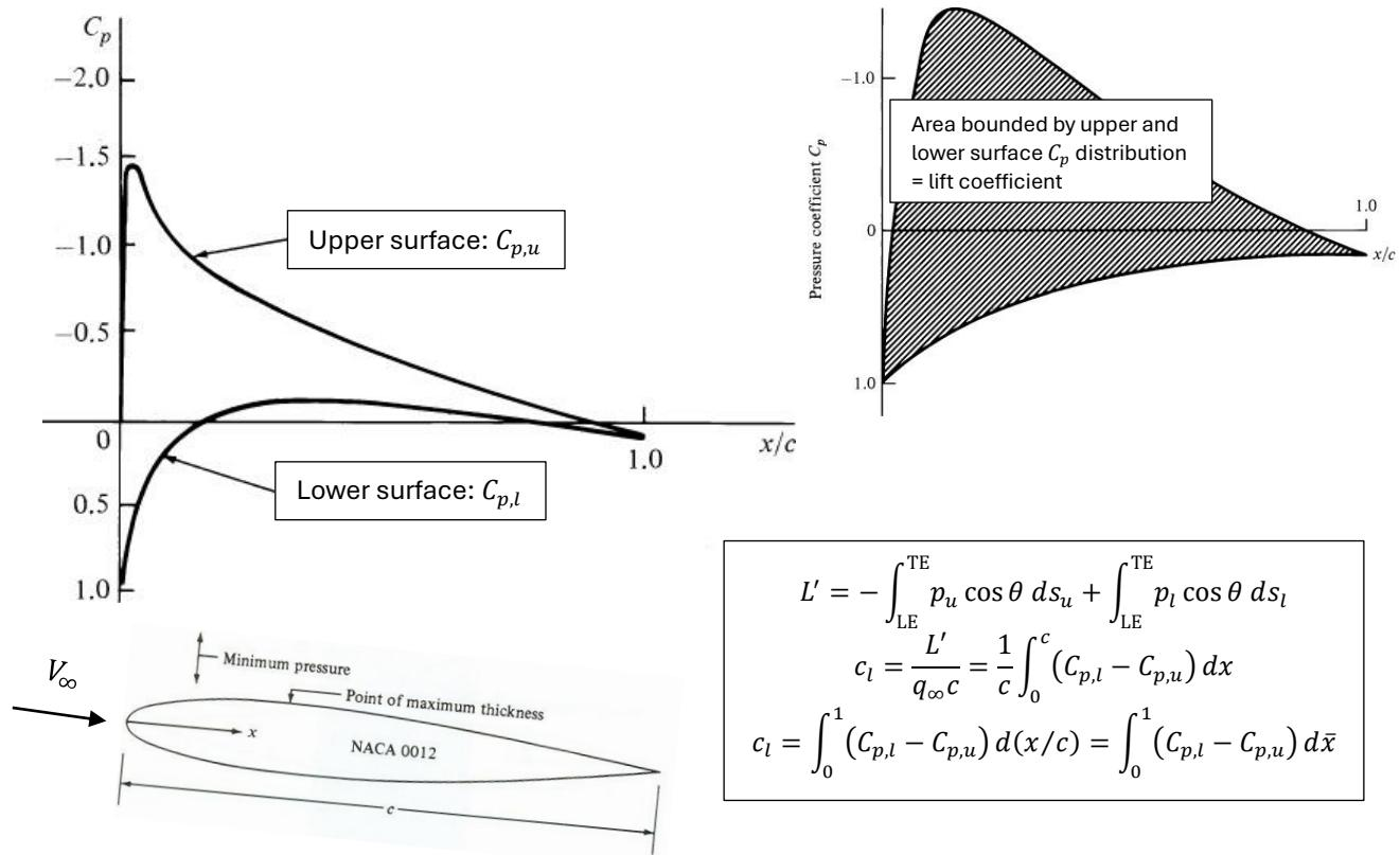
Pressure coefficient plot and lift coefficient (source: J.D. Anderson "Fundamentals of Aerodynamics" 2016)
