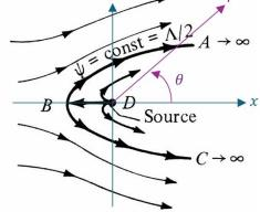
Potential flow field simulation (source: J.D. Anderson "Fundamentals of Aerodynamics" 2016)
