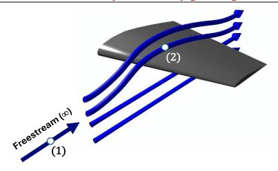
Consider an aircraft wing in a flow of air, where far ahead upstream of the wing (called a **freestream**), the pressure, velocity, and density are measured as: 1 atm (standard sea-level), 100 mph, and 0.0024 slugs/ft<sup>3</sup>, respectively. At a given point on the wing, the measured pressure is 2,070 lb/ft<sup>2</sup>. What is the velocity at this point?
